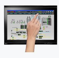
IP65 rating, and is even protected against dust and hose water getting into it. Other properties: A special coating protects the electronics from moisture. And the ventilator of the monitor can be accessed easily for a simple replacement.
