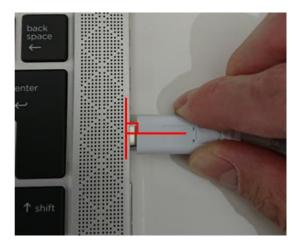
Please note that the cable or PC may be damaged if it is plugged in or unplugged in the following ways.
